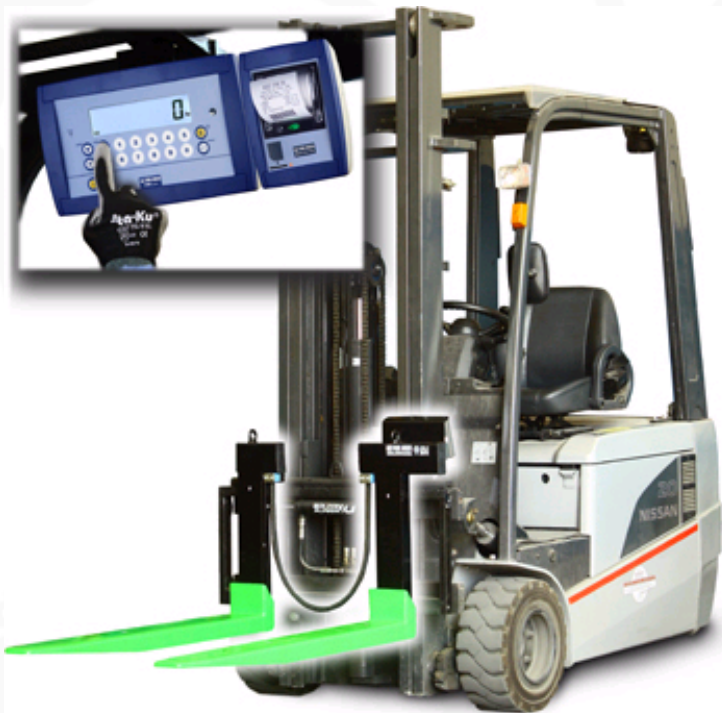
LTF: pair of weighing forks. Indicator for mounting in the cabin, with optional printer.
